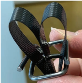
Feed the loops through the large wire square hole.
