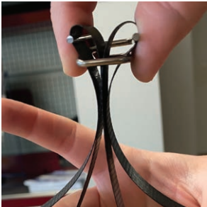
Position the loops on each side over the wire buckle end pins.
